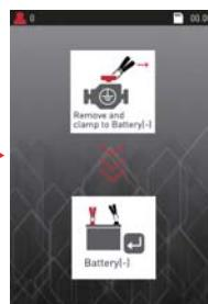
This screen indicates that the negative clamp must be attached back onto the battery's negative terminal
