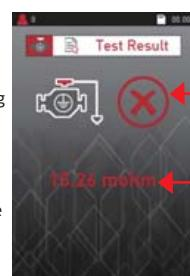
Test result indicating the ground connection is not good.
